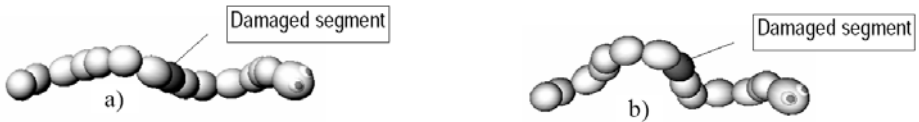
Fig. 6.16. The frontal view of the Snakebot before (a) and after the adaptation (b) to the damage of a single segment. The corresponding views from above of the sidewinding Snakebot are shown in Fig. 6.15a and b, respectively.
