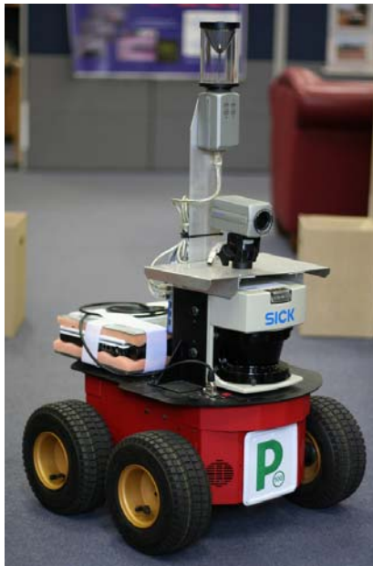
Fig. 5.2. Typical mobile robot equipped with a bearing-only sensor (panoramic camera).
